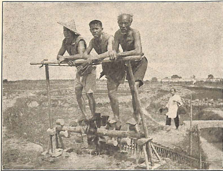
Pumping water from irrigation ditch into rice fields, South China
