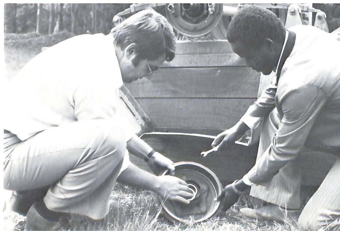
(Left) Throughout the daily work and activities at the school, there is always need for College upkeep, maintenance, and repairs, for which Missionary Ken Priebe is responsible. Ken and student repair a wheel bearing on the trailer.
