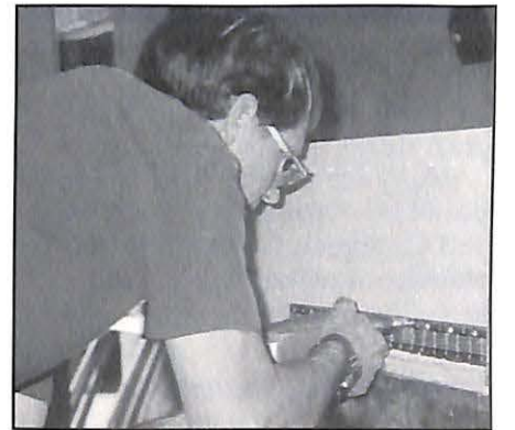
Ken Soulès makes a makeshift jig for adjustable cabinet shelves.
